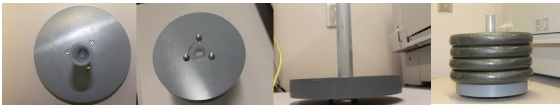
Figure 6. Point loading calibration device
